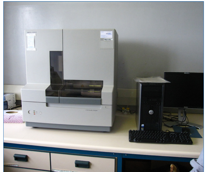
Figure 4.5: HIV Genotyping: A 3130 Genetic Analyser at the National Microbiology Reference Laboratory, Harare, Zimbabwe
