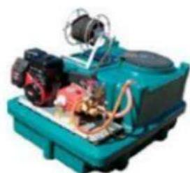
Slip-on unit suitable for single or double cab L.V.
