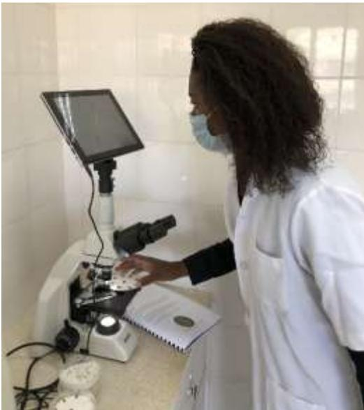
*1. Binocular Optical Microscope allows for greater speed in the identification of phyto-pathogenic species.*
