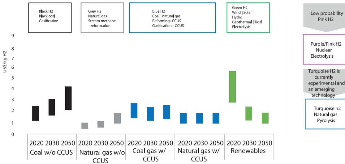
**Figure 15:** Levelised Cost of Hydrogen Production by Technology In 2020, and in the Net Zero Emissions Scenario, 2030 And 2050 <sup>13</sup>.
