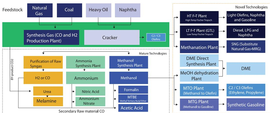
**Figure 11:** Petrochemical Production from Various Input Sources
